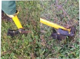
Now comes The Popper. The AR team provides us with three fantastic garish yellow and black jobs. You plonk the tool so that it grips a low lying hawthorn bush, tighten the hold on the stem and lever back on to the base plate. Mirabile dictu. The whole thing comes away root as well ready to be tossed on the collection pile.
